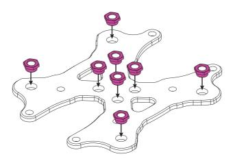
Take a big screw and insert the locknuts one by one.
